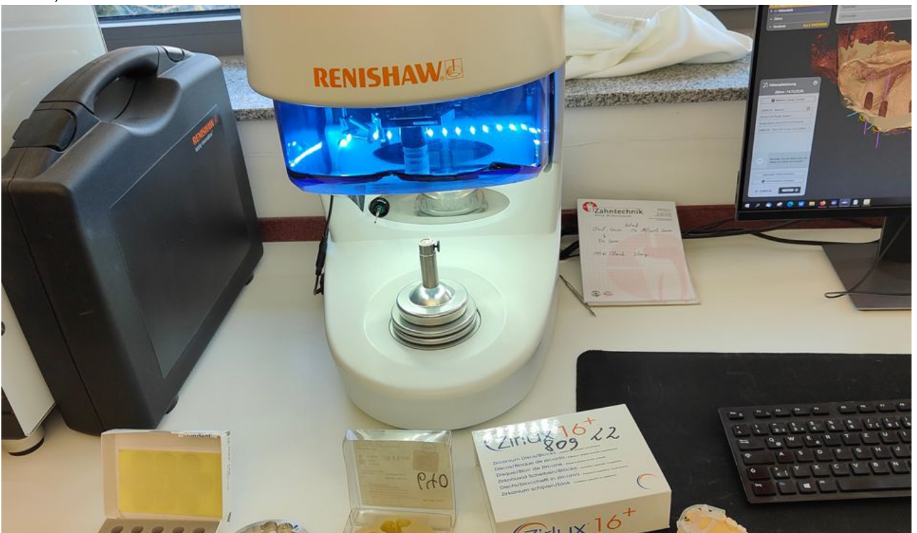
« Zurück Optical and tactile dental scanner that detects the position and alignment of the dental model and implants (Bild 6 von 7) » Vorwärts
